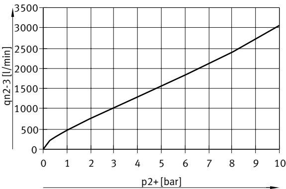
Flow rate q_n from 2 -> 3 as a function of excess output pressure p_2 , VPPM-8L/F-...-0L10H-... (10 bar)
