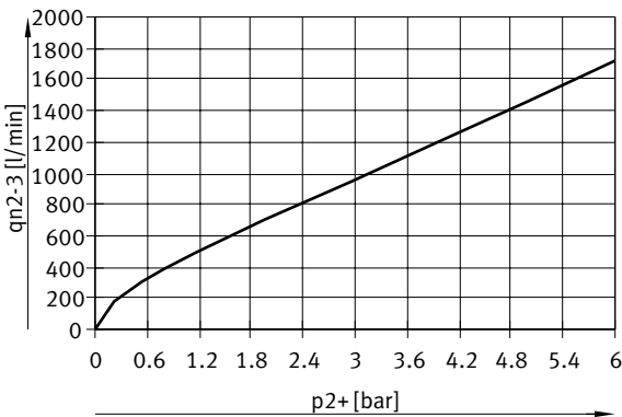
Flow rate q_n from 2 -> 3 as a function of excess output pressure p_2 , VPPM-8L/F-...-0L6H-... (6 bar)
