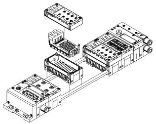
The CPX modules are mechanically connected to each other using tie rods. The entire unit can be assembled using two screws in the end plates. The tie rod ensures that the unit has a high mechanical load bearing capacity and is therefore the mechanical backbone of the CPX terminal.
