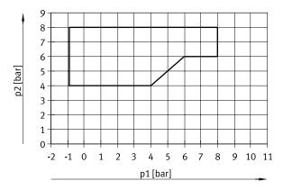
For valves in valve size 10 mm with code for position function 1-32: MU, NU, KU,  $\,\mathrm{HU}$
