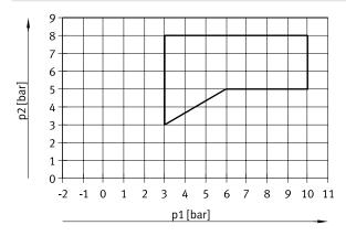
For valves in valve size 14 mm with code for position function 1-32: MS, NS, KS, HS, DS  $\,$
