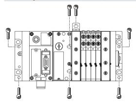
The valve terminal MPA-L is screwed onto the mounting surface using four M4 and two M6 screws or using six M6 screws. The mounting holes are on the left and right end plates and in the pneumatic interface.
