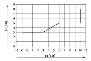
For valves in valve size 10 mm with code for position function 1-32: MS, NS, KS, HS, DS  $\,$
