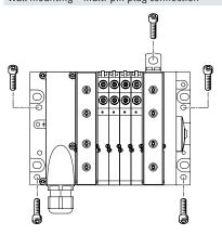
The valve terminal MPA-L is screwed onto the mounting surface using four M4 or M6 screws. The mounting holes are on the multi-pin plug connection and on the right end plate.
