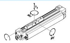
If the drive is subjected to two or more of the indicated forces and torques simultaneously, the following equatio must be satisfied in addition to the indicated maximum loads:
