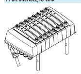
I-Port/IO-Link® consists of a central master and the I-Port interface/IO-Link® devices connected via special connecting cables. This permits a decentralised layout of the devices. The connection type corresponds to a star topology.
