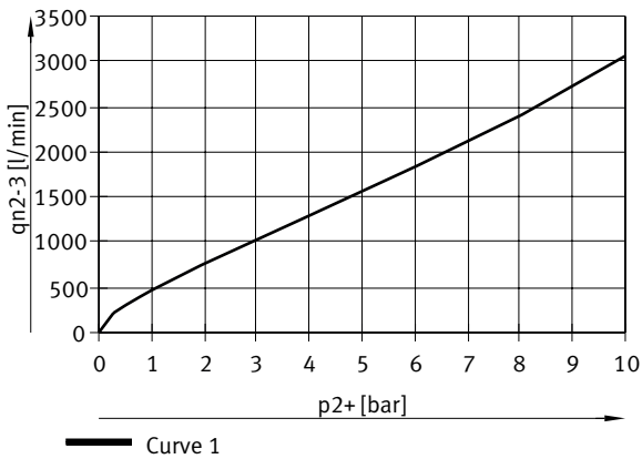
Flow rate q_{n2-3} from 2 -> 3 as a function of excess output pressure p_{2+} , VPPM-8L/F-...-0L10H-... (10 bar)
