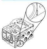
MPA offers a number of options for creating pressure zones if different working pressures are required. Depending on the electrical interface, up to 16 pressure zones are possible.
