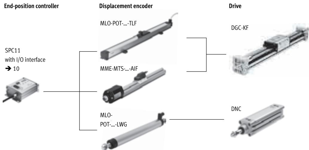
With external/integrated displacement encoder
