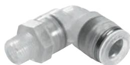
Polypropylene fitting for use in applications with extreme media influences. For pneumatic applications with a temperature range up to 60°C and a pressure range up to 10 bar. Tubing O.D. 4, 6, 8, 10 and 12 mm with connecting threads R1/8 ... R1/2.
