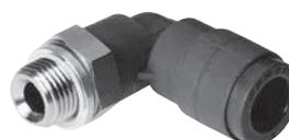
Flame-retardant push-in fitting for use in all areas where there is a risk of fire, for example welding systems in the automotive industry, and in the construction industry. For pneumatic applications with a temperature range up to 60°C and a pressure range up to 10 bar. Tubing O.D. 4, 6, 8, 10 and 12 mm with connecting thread R1/8 ... R1/2 and G1/8 ... G1/2.
