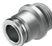
Stainless steel push-in fitting. Maximum corrosion resistance CRC 4 and chemical resistance. For pneumatic applications with a temperature range up to 150°C and a pressure range up to 16 bar. Tubing O.D. 4, 6, 8, 10, 12, 14 and 16 mm with connecting thread M5, M7 and G1/8 ... G1/2.
