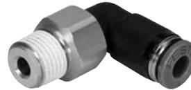
Push-in fitting with swivel joint, rotatable 360°. The ball bearing enables rotating movements in the application up to max. 500 rpm. For pneumatic applications with a temperature range up to 60°C and a pressure range up to 14 bar.
