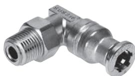
Stainless steel push-in fitting. Maximum corrosion resistance CRC 4 and chemical resistance with approval for use in the food and packaging industry. For pneumatic applications with a temperature range up to 120°C and a pressure range up to 10 bar. Tubing O.D. 4, 6, 8, 10, 12 and 16 mm with connecting threads M5 and R1/8 ... R1/2.
