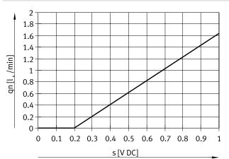
Formula for calculating the setpoint value s as a function of the required nominal flow rate
