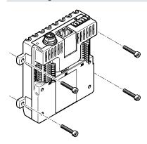
Sturdy wall mounting of the valve control module using four through-holes.
