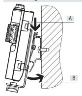
The H-rail mounting VAME-V3-H consists of a mounting bracket and a clamp:
