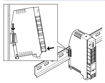
The module is attached to the H-rail or the electrical manifold module and latched in place.
