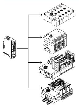
The IO-Link master module provides 4 external IO-Link interfaces.
