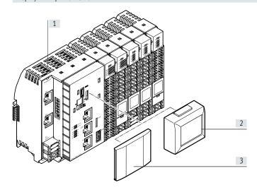
The operator unit CDSB-A1 from Festo is a plug-in display and operating panel for the automation system CPX-E.
