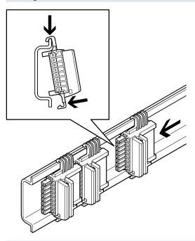
The electrical manifold modules are clipped into the H-rail. They can be moved along the H-rail.
