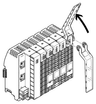
A hinged identification holder is available for the input and output modules and IO-Link master modules.
