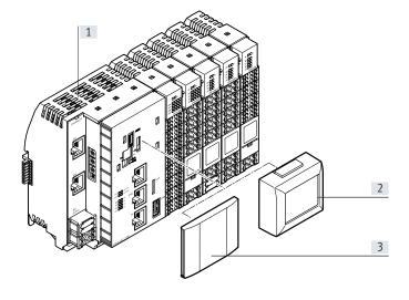
The operator unit CDSB-A1 from Festo is a plug-in display and operator unit for the automation system CPX-E.
