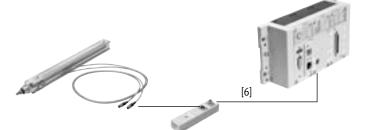
• The measuring signal of the linear drive DNCI is an incremental signal. This signal is converted to a CAN signal in the sensor interface CASM-S-D3-R7. The converted signal is then read into the CPX-CMIX module
