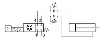
The travel time for retracting and advancing is preset in the Motion Terminal VTEM.
