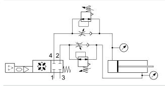
The required setpoint value can be independently preset for ports 2 and 4. The Motion Terminal VTEM autonomously regulates the pressure and signals the actual pressure in ports 2 and 4 and to the higher-order controller.
