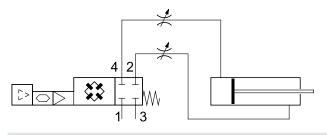
The flow rate can be individually adjusted for each port; the supply air and exhaust air flow control are adjusted independently of one another.
