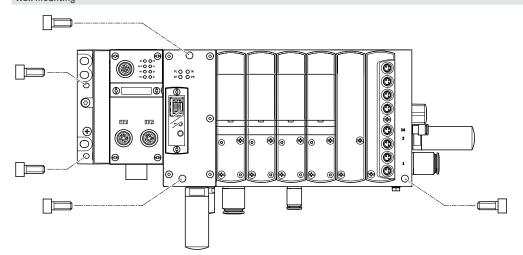
The Motion Terminal VTEM is screwed to the mounting surface using five M4 or M6 screws.
