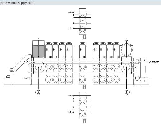
External pilot air supply, right-hand end plate without supply ports
