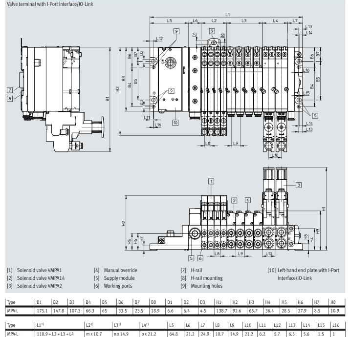
1) m, n, o = number of sub-bases/valve positions (m = width 10 mm, n = width 14 mm, o = width 20 mm)
