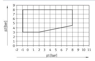
For valves in width 14 mm with code for position function 1-32: MS, NS, KS, HS, DS  $\,$
