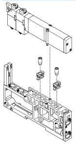
Cover plate (code L) without valve function, for reserving valve positions on a valve terminal. Valves and cover plates are attached to the sub-base using two screws.
