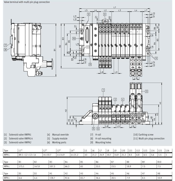
1) m, n, o = number of sub-bases/valve positions (m = width 10 mm, n = width 14 mm, o = width 20 mm)
