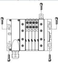
Wall mounting - Fieldbus interface (CPX terminal)
