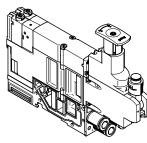
Additional functional units can be added to each valve position between the base plate and the valve. These functions are known as vertical stacking modules and enable special functions or control of an individual valve position.
