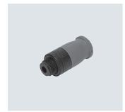
Plastic fitting for easy installation with one-hand operation. Hydrolysis-resistant, FDA-compliant and easy to clean. For pneumatic applications with a temperature range up to 60 °C and a pressure range up to 10 bar. Tubing 0.D. of 6 mm with connecting thread G1/8.
