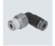
Push-in fitting with swivel joint, rotatable by 360°. The ball bearing enables rotating movements in the application up to max. 500 rpm. For pneumatic applications with a temperature range up to 60 °C and a pressure range up to 14 bar.
