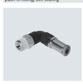
Push-in fitting that blocks the air flow after the tubing is disconnected. For pneumatic applications with a temperature range up to 60 °C and a pressure range up to 14 bar.
