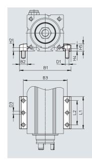
• For mounting the axis on the side of the profile. The profile mounting can be attached to the mounting surface using the drill hole in the centre.
