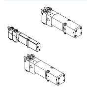
VMPA offers a comprehensive range of valve functions. All valves have a patented sealing system, which ensures efficient sealing, a broad pressure range and a long service life. They have a pneumatic pilot control for optimising performance. Compressed air is supplied via a pilot air supply port.
