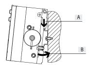
The MPA-L valve terminal is attached to the H-rail (see arrow A).
