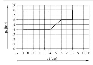
For valves in width 20 mm with code for position function 1-32: MS, NS, KS, HS, DS  $\,$
