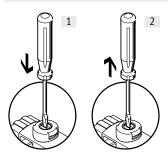
Press in the stem of the MO with a pointed object or screwdriver.
