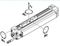
If the drive is subjected to two or more of the indicated forces and torques simultaneously, the following equation must be satisfied in addition to the indicated maximum loads:
