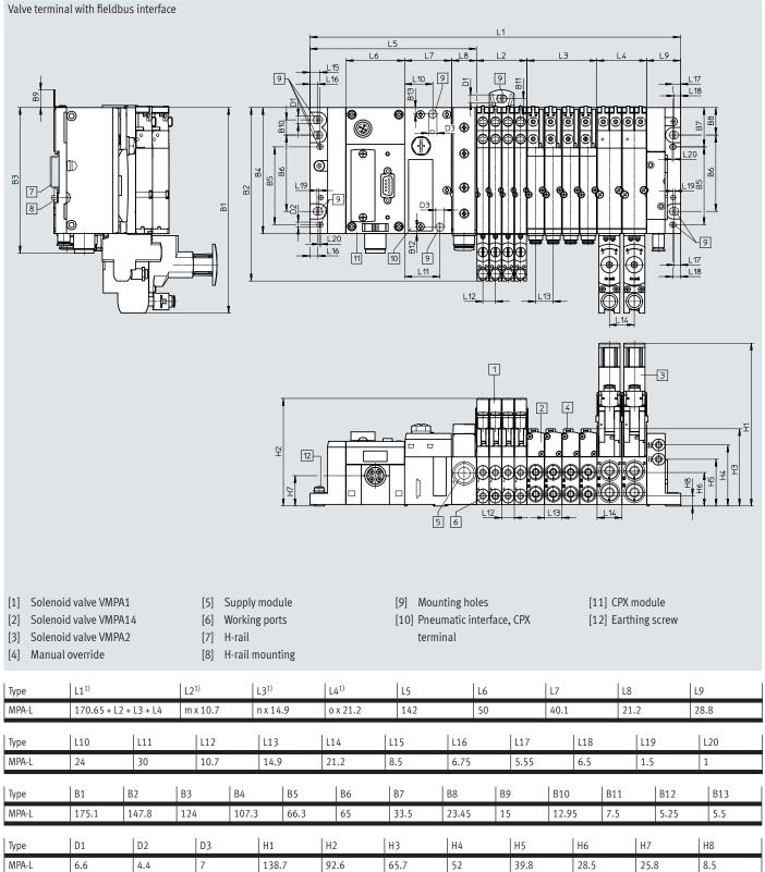
1) m, n, o = number of sub-bases/valve positions (m = width 10 mm, n = width 14 mm, o = width 20 mm)
