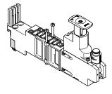
An adjustable pressure regulator can be installed between the base plate and the valve to control the force of the actuator. This pressure regulator maintains a constant output pressure (secondary side) independent of pressure fluctuations (primary side) and air consumption.
