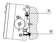
onto the mounting surface using four M4 and two M6 screws or using six M6 screws. The mounting holes are on the left-hand and right-hand end plate and on the pneumatic interface. Optional mounting brackets are also available.
