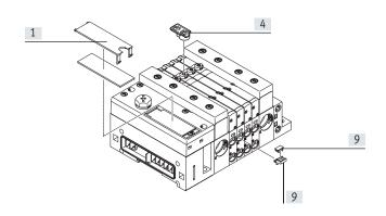
A holder VMPAL-ST-AP-10 (part no. 561109) with inscription labels (part no. 18576, IBS-6x10) can be mounted on each sub-base for labelling the valves. The inscription label holder ASLR-D-L1 can be pushed onto the manual override.
