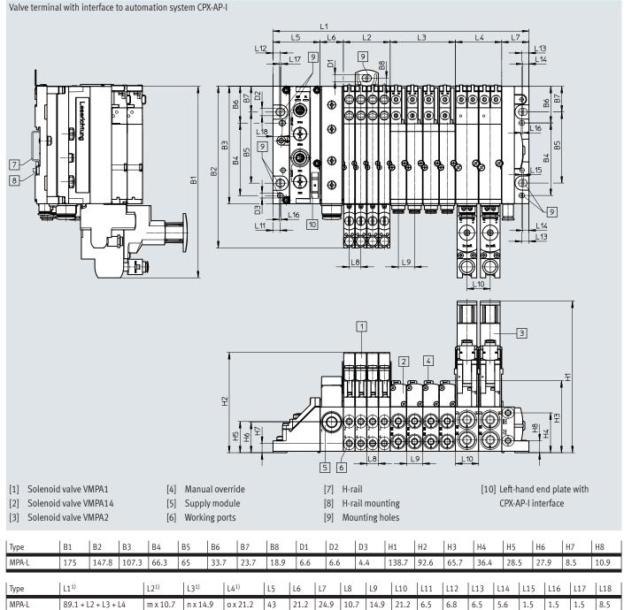
1) m, n, o = number of sub-bases/valve positions (m = width 10 mm, n = width 14 mm, o = width 20 mm)
