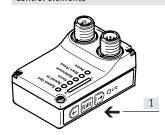
[1] Pushbuttons for parameterisation and control
