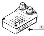
[1] Pushbutton actuators for parameterisation and control
