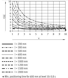
→ Max. speed level for payload: level 10
