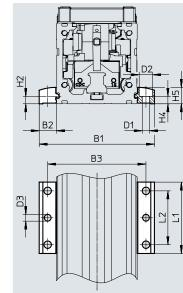
• For mounting the axis on the side of the profile. The profile mounting can be attached to the mounting surface using the drill hole in the centre.
