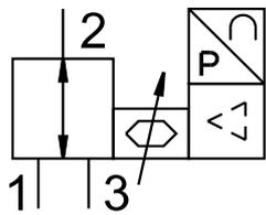
An integrated pressure sensor records the pressure at the working port and compares this value with the setpoint value.
