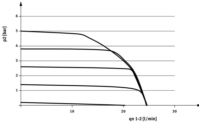
Flow rate  $q_n$  from 2 → 3 as a function of output pressure  $p_2$
