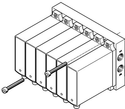
The manifold rail also has through-holes for wall mounting.
