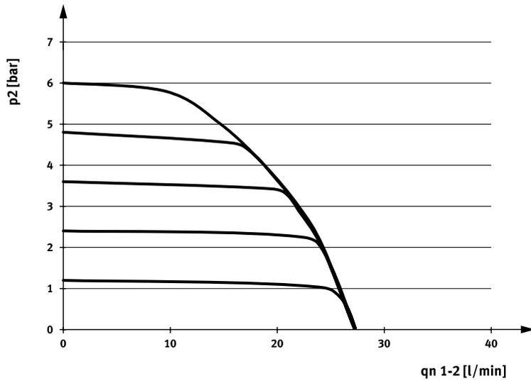
Flow rate  $q_n$  from 2 → 3 as a function of output pressure  $p_2$
