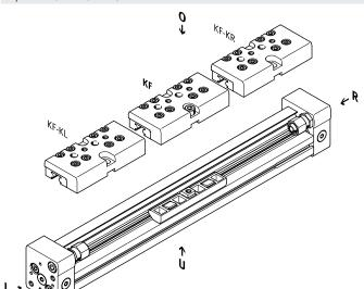
GP – With protected recirculating ball bearing guide
