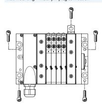
The MPA-L valve terminal is screwed onto the mounting surface using four M4 or M6 screws. The mounting holes are on the multi-pin plug connection
