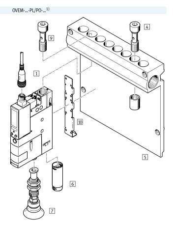
1) Hollow bolt 🖸 and mounting bracket 10 are included in the scope of delivery of the OVEM-...-PL/PO-....
