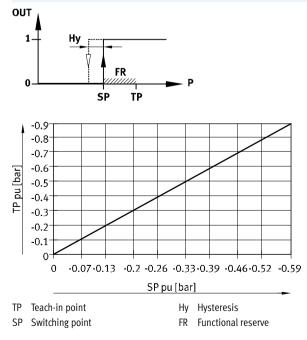
If the desired threshold value 1 for the vacuum is reached, vacuum generation is automatically switched off. A check valve prevents a decrease of the vacuum.
