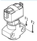
Theoretical actuating force due to stroke compensation for design variant with stroke compensation.
