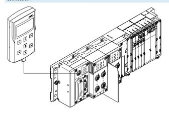
The operator unit is connected to the CPX-P terminal using pre-assembled cables.
