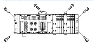
The end plates of the CPX-P terminal, the valve terminal and the pneumatic interface include mounting holes for wall mounting. Additional mountings for the CPX-P terminal are available for longer valve terminals.
