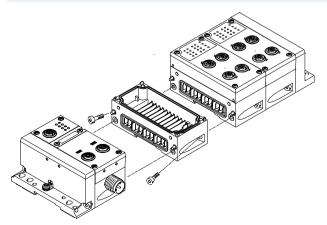
The mechanical connection between the CPX-P modules is created using special angle fittings. The CPX-P terminal can thus be expanded at any time. Key features – Power supply
