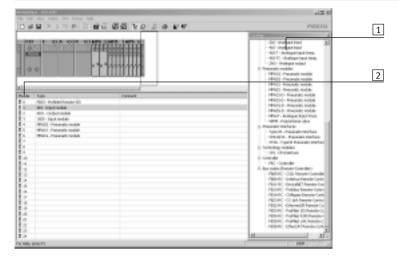
The device configuration can be conveniently generated, parameterised and saved using the drag & drop feature. You can insert and move modules.
