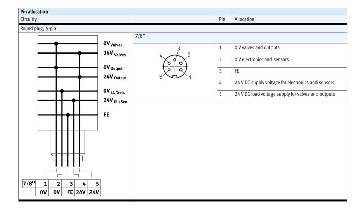
**Terminal CPX-P**Technical data – Interlinking block with system supply
