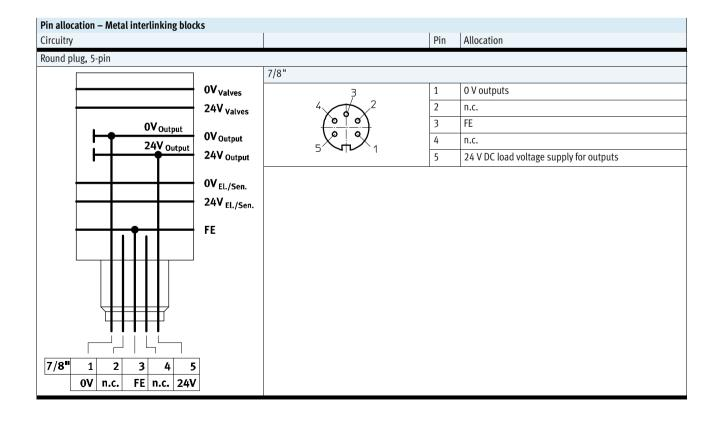
**Terminal CPX-P**Technical data – Interlinking block with additional power supply for outputs
