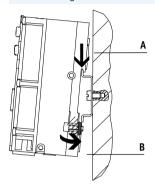
The rear profile of the CPX-P interlinking block has a preformed H-rail mounting so that the CPX-P terminal can be attached to the H-rail using the H-rail mounting kit.
