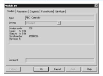
Displays important module data as well as the number of allocated inputs and outputs.
