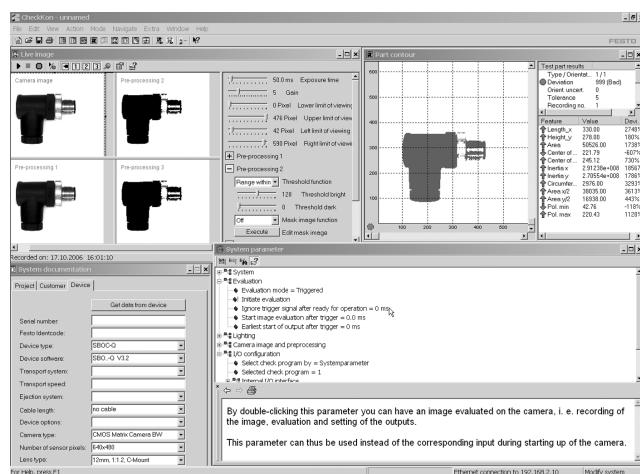
Using the CheckKon software, all processes within the camera – from image capture to the input and output parameters – can be displayed, logged and modified.
