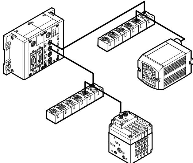
– The Compact Vision System SBO...-Q can be integrated into a Festo CPI network. In this case it functions like a binary module with 16 inputs and outputs.
