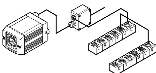
An input and output module can be connected to the camera via the camera's CAN interface.
