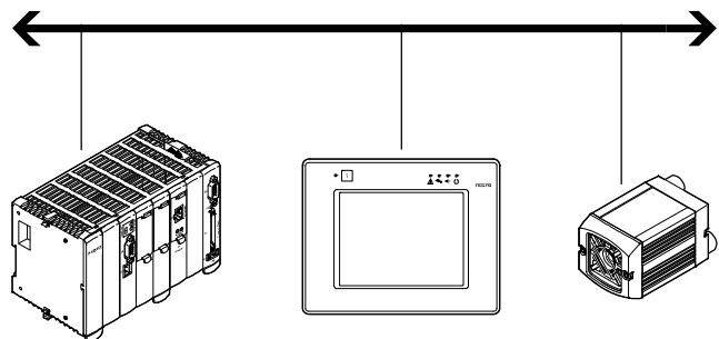
All parameters can be modified and all inspection results and characteristic values can be read via the Ethernet interface with EasyIP, Telnet and Modbus TCP.
