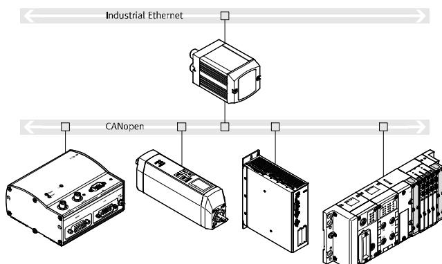
Servo controllers and remote I/O can be addressed directly via the CANopen master functionality.
