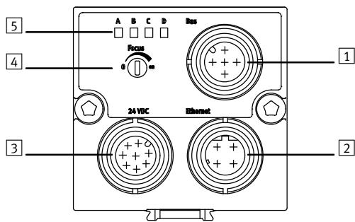
**1** Fieldbus connection for Compact Vision Systems SBO...-Q-R1 and SBO...-Q-R2
