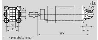
1 The pivot pin is secured against rotation with a dowel pin.
