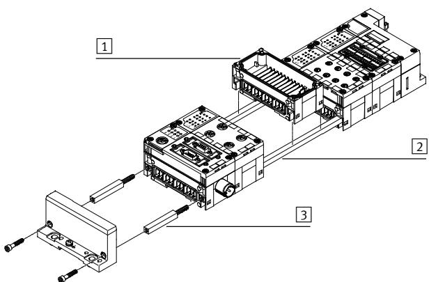
The mechanical connection between the CPX modules is created using special tie rods [2]. Two screws in the end plates are all that are needed to assemble the entire unit. The tie rod ensures that the unit resists high mechanical loads and is therefore the “mechanical backbone” of the CPX terminal.
