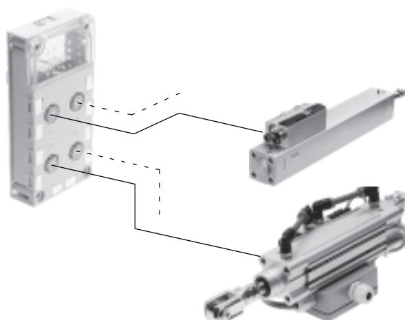
Since the module supports the M12 connection block (8-pin), up to 4 cylinder/valve combinations with integrated sensors can be connected. Each cylinder/valve combination is supported by 2 inputs and 2 outputs per socket. It is therefore possible to control max. 2 solenoid coils and record signals from 2 sensors with a pre-assembled cable.
