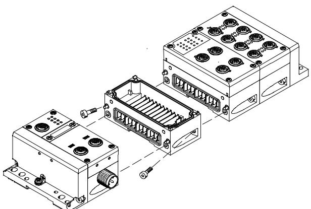
The mechanical connection between the CPX modules is created using special angle fittings. The CPX terminal can thus be expanded at any time.
