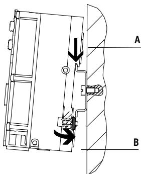
The H-rail mounting is formed in the reverse profile of the CPX interlinking blocks. The CPX terminal can be attached to the H-rail using the H-rail mounting kit. The CPX terminal is mounted on the H-rail (see arrow A) and
