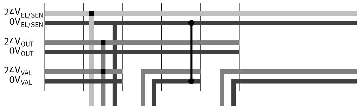
The use of decentralised devices on the fieldbus – particularly with high protection for direct machine mounting – demands a flexible power supply concept. A valve terminal with CPX can, in principle, supply all voltages via a single socket.
