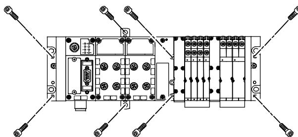
The end plates of the CPX terminal, the valve terminal and the pneumatic interface include mounting holes for wall mounting. Additional mountings for the CPX terminal are available for longer valve terminals. These mountings differ depending on the design of the CPX terminal (plastic or metal).
