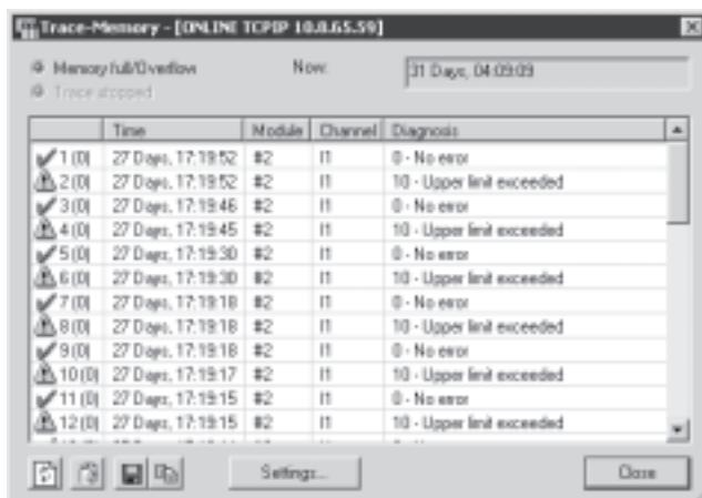
Faults which occur during operation are entered in a diagnostic memory. The first or the last 40 entries are saved, as well as the respective time measured from the moment the power supply was switched on.
