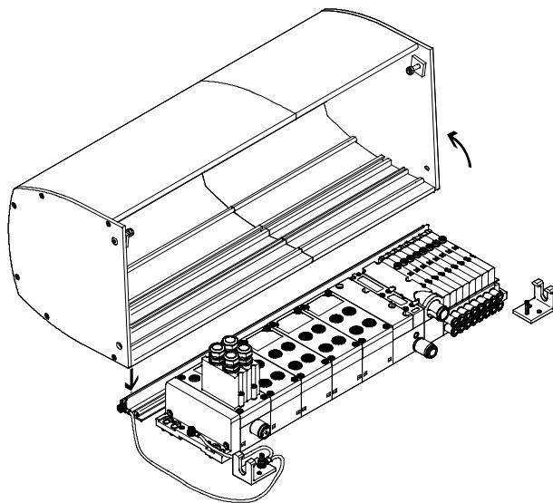
The CPX hood CAFC is a space and cost-saving alternative to a control cabinet. It is designed as an extruded aluminium profile and is installed on a mounting plate. The valve terminal (CPX with MPA-S or MPA-L) is well protected and is quick to install without the need for complex control cabinet installation for cables and tubing.
