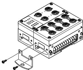
Additional mounting brackets for the CPX terminal that can be screwed onto the interlinking blocks are available for longer valve terminals.
