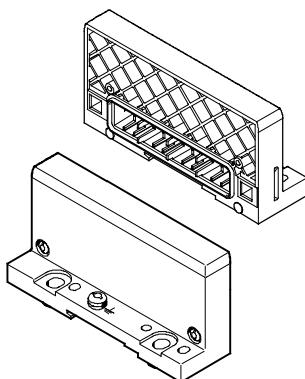
Earthing plate (for end plate for plastic design)
