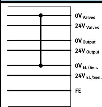
The module combines the 0 V potential of the power supply for electronics and sensors with the 0 V potential of the power supply for valves.
