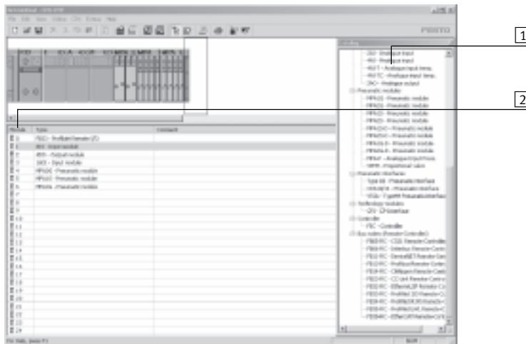
The device configuration can be conveniently generated, parameterised and saved using the drag & drop feature. You can insert and move modules.
