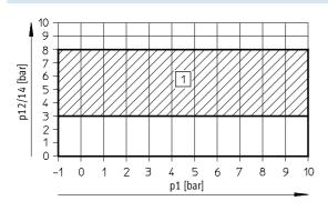
Switch-on pilot pressure of 3/2-way valves
