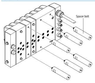
The CDVI can be mounted directly on earthed mounting surfaces using the four threaded holes in the basic block and the spacer bolts ordered via the order code (accessories order code Y).
