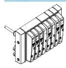
Control signals from the controller to the valve terminal are transmitted via a pre-assembled multi-wire cable or a self-assembly multi-pin plug connection, which substantially reduces installation time. Valve terminals with multi-pin plug connections can be equipped with 4 to 16 valve positions with max. 24 solenoid coils.
