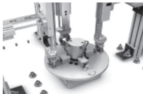
Rotary table with stationary centre section
