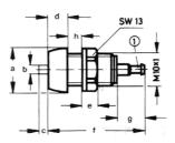
1 Barbed fitting for 3 mm tubing SW = wrench size, mm
