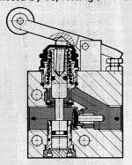
Full free flow through the check valve is independent of initial roller lever position.
