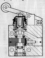
In Type GGO, the needle valve is gradually closed by depressing the roller lever.
