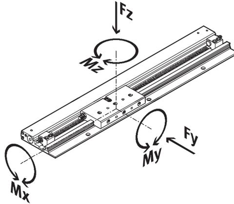
If the drive is subjected to several of the indicated forces and torques simultaneously, the following equations must be satisfied in addition to the indicated maximum loads:
