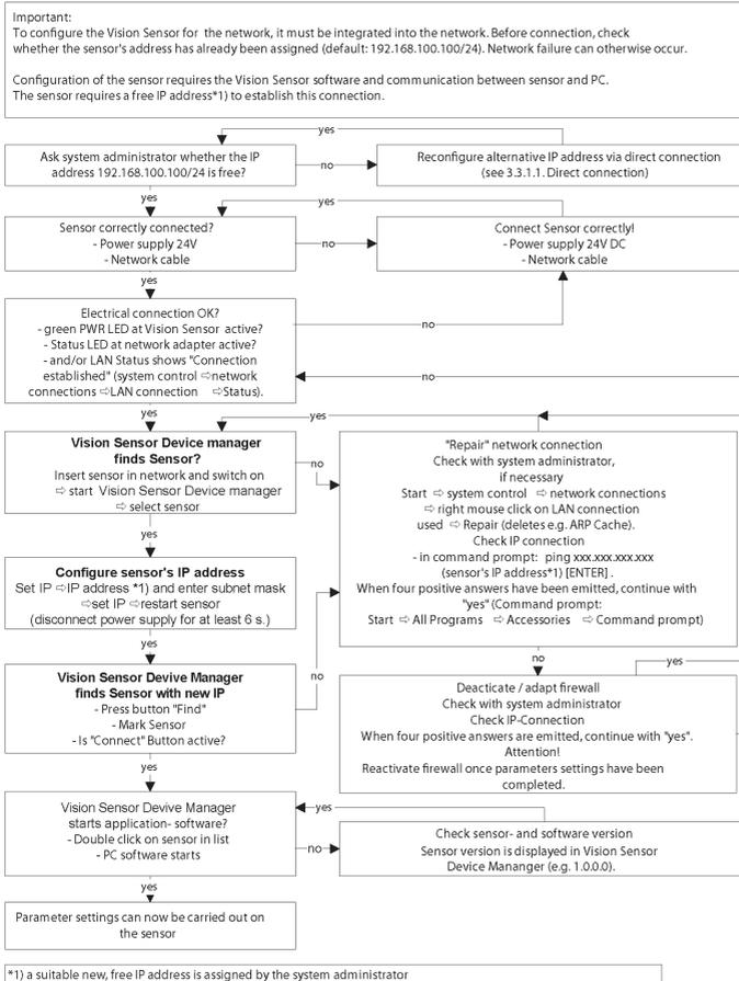
Fig. 2: Connection via network sensor / PC, procedure and troubleshooting
