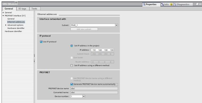
Fig. 32: Configuring the IP address in the project
