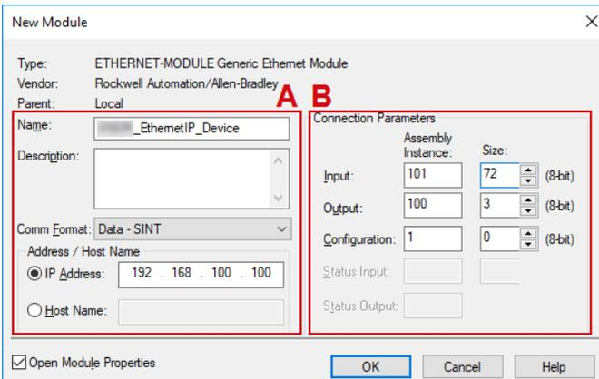
Fig. 59: Assignment of the device name and IP address
