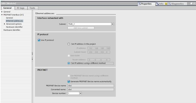
Fig. 33: Configure the IP address for the SBS in Vision Sensor Device Manager; the corresponding settings can be found in the PLC/TIA interface
