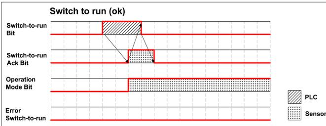
Fig. 25: Timing Switch to run ok
