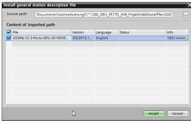
Fig. 28: Selecting and installing the GSD file
