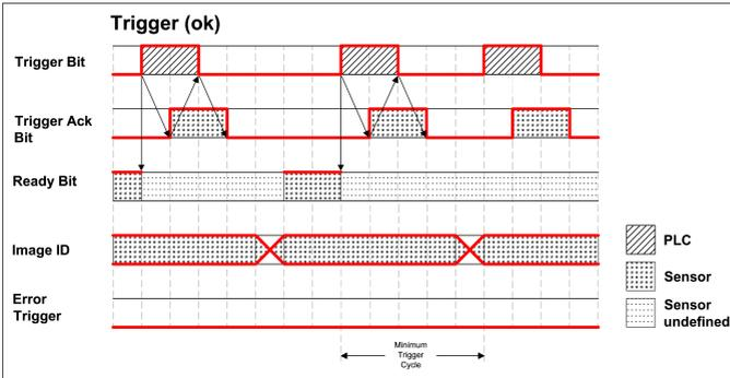
Fig. 20: Timing Trigger ok
