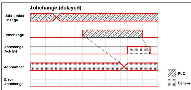
Fig. 23: Timing Job change delayed
