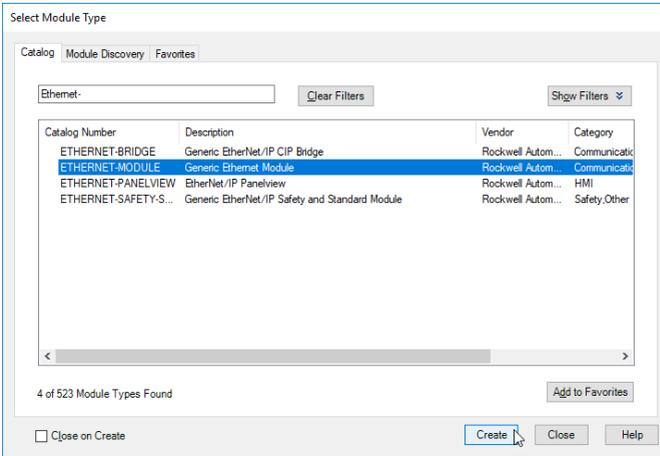
Fig. 58: Selection of "Generic Ethernet Module"
