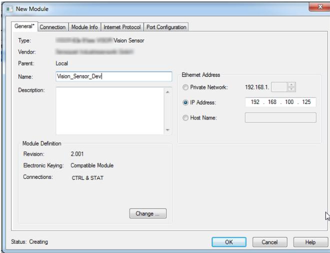
Fig. 55: Configure the device name and IP address
