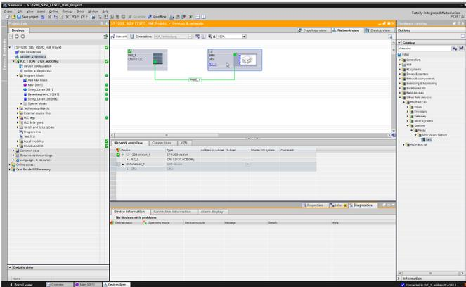
Fig. 30: Connecting the SBS to the PLC
