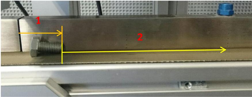
Figure 3.1 shows an example of the situation. The distance 1 describes the position after the scanning process and the calculation time. The distance 2 describes the space to possible discharge position. The distance 2 must never be smaller than 1 mm!
