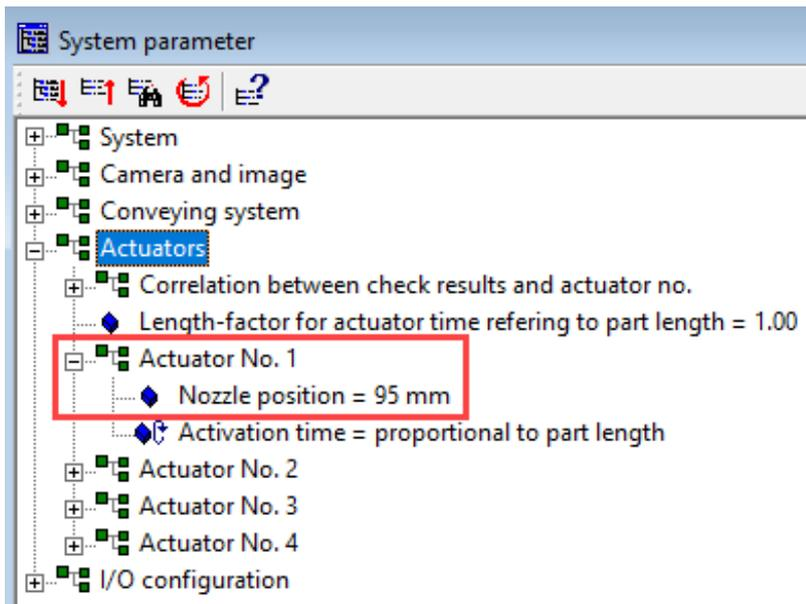
When using valves to blow off parts, the setting "Activation time = proportional to part length" must be set. (default value)
