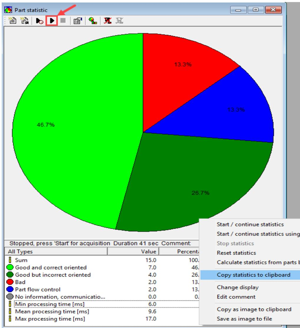
The blue "pie" represents the parts, that have been ejected by the part flow control. This includes parts, that were fed during jam sensor was active or in counter mode, when the preset counter value is reached.
