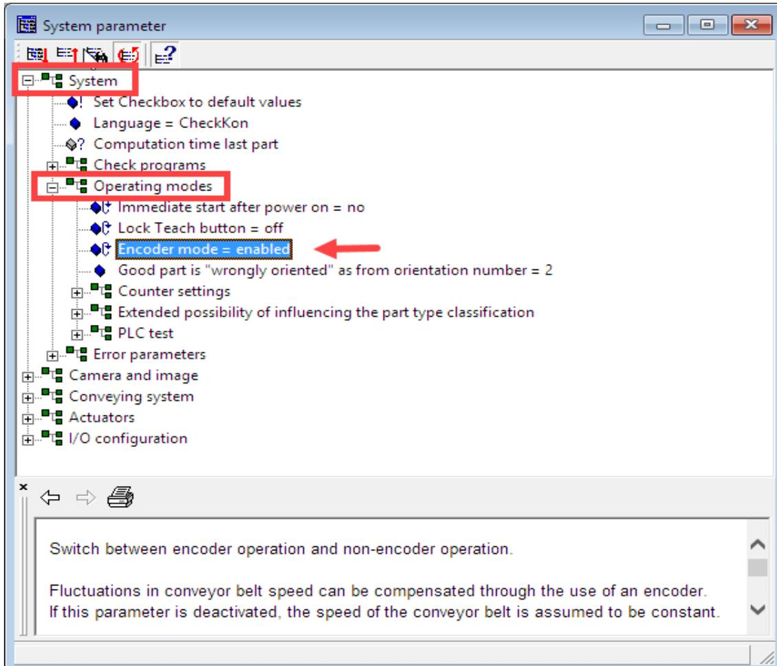
Here, the encoder can be enabled or disabled via a toggle function. Make the selection according to the existing system.
