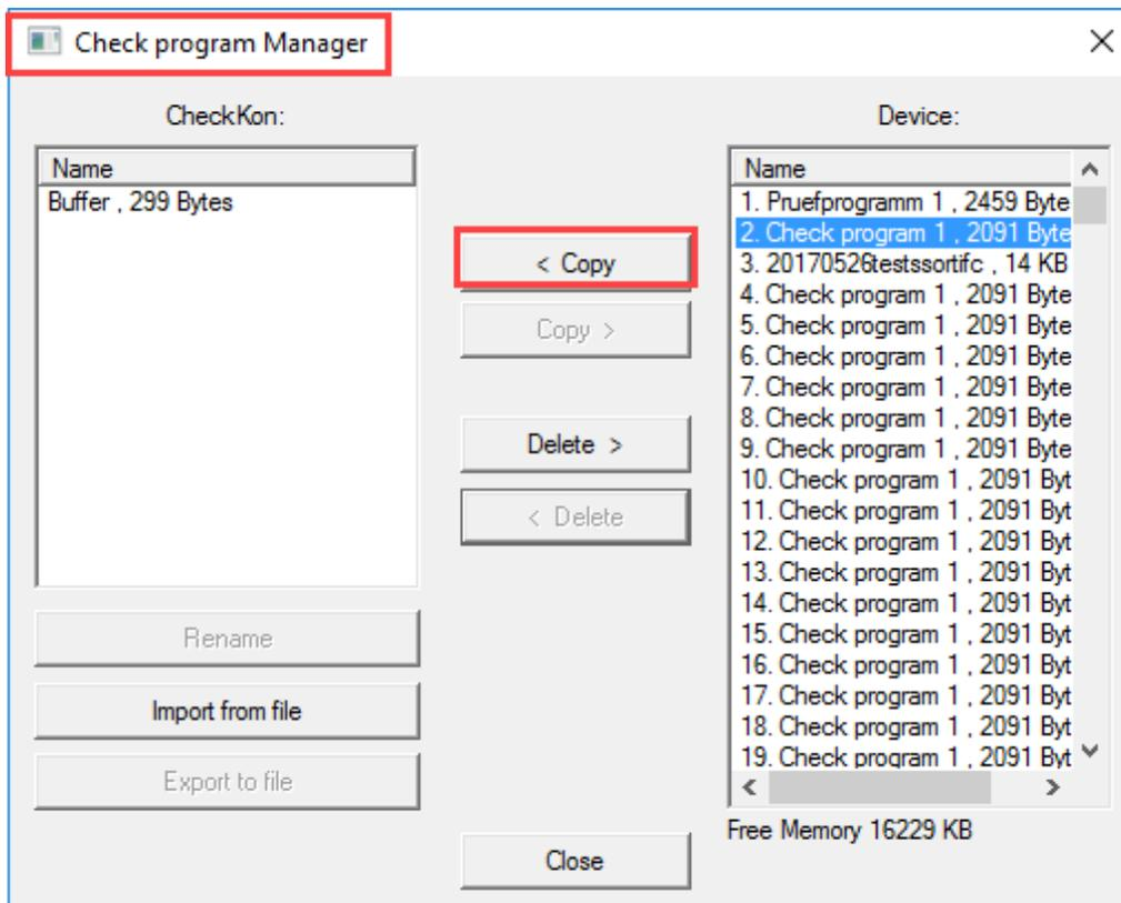
Mark the memory locations with the taught-in parts in the "Device" column on the right-hand side. Then press the "< Copy" button.
