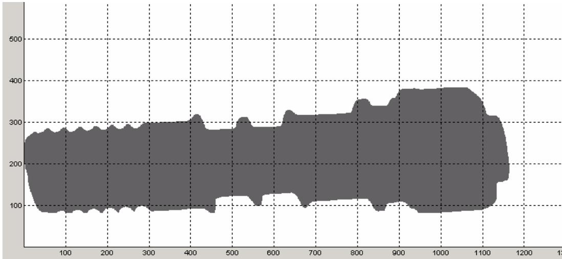
Note: with the slider "Change scaling of axis" the display can be adapted to the real appearance of the parts. This does not change the resolution, only the representation of the image on the screen!
