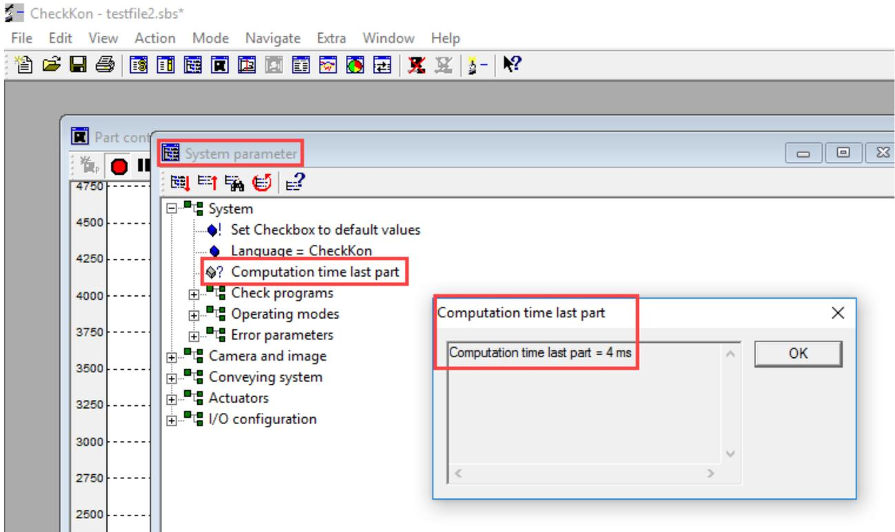
The dialogue window shows the required processing time. It includes also the duration of the data/image transmission to the connected PC.
