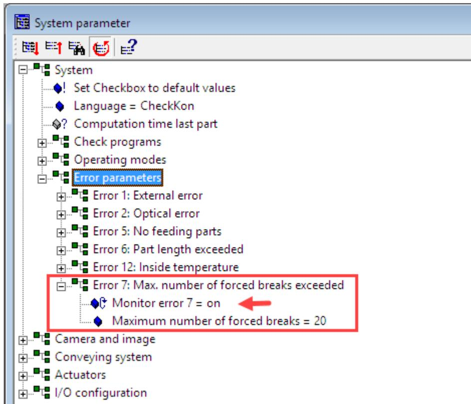
When the maximum number of forced breaks is reached, an error Error 7 is generated and the system stops.
