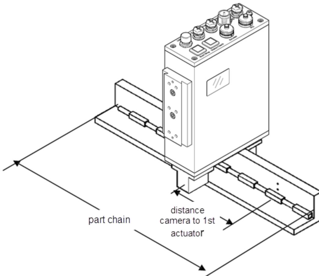
To prevent this situation, the parameter "Forced stop of analysis =" is used. This causes that the analysis will be interrupted and a new scan is started. The point of interruption is adjusted by the mm-value in the parameter "Maximum part length". This causes several "artificial parts" which were discharged accordingly to the parameter setting of actuators.
