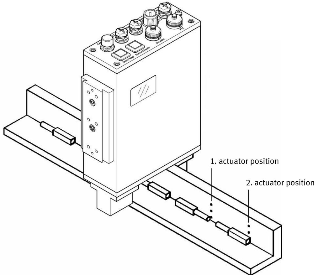
According to the categories, this configuration with 2 discharge positions represents the minimum configuration. Even if no bad parts are to be expected, there is a possibility that the Checkbox will come to a negative result. Possibly caused by poor feeding or non-optimal test settings. These parts are then sorted out at the bad part position.
