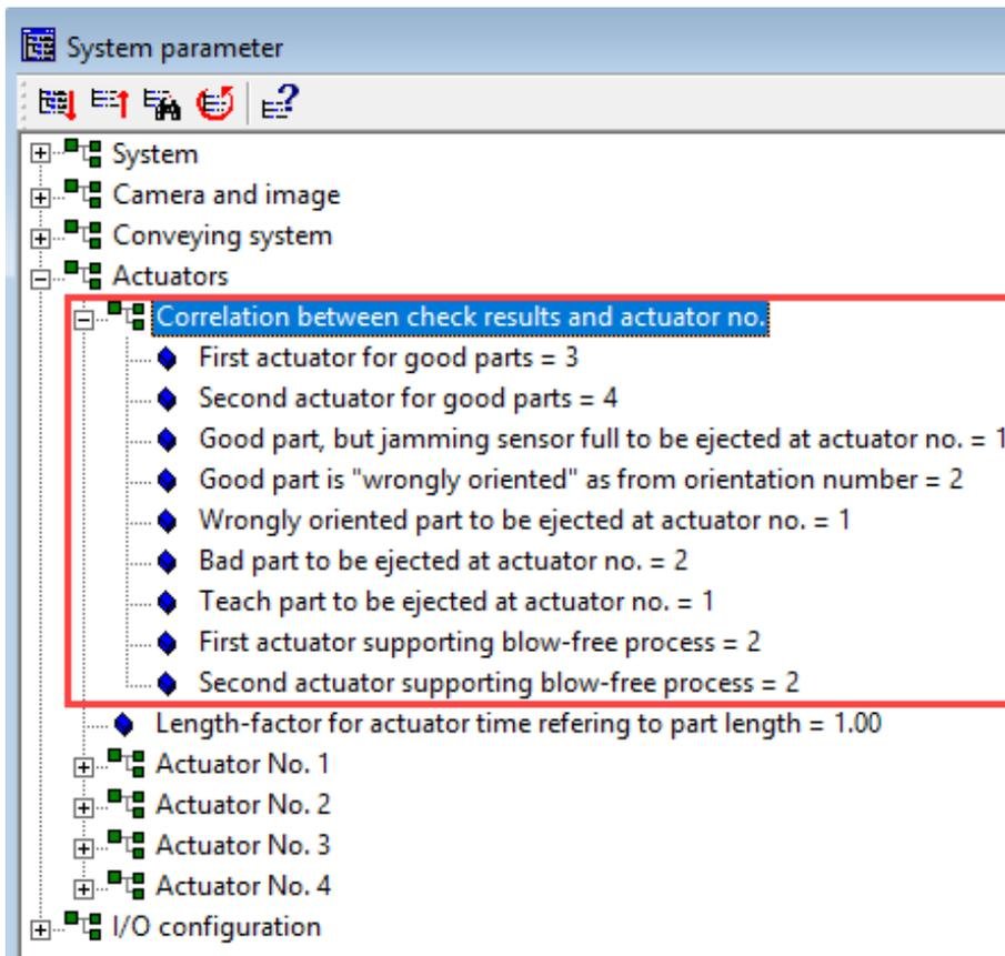
Each category of parts is assigned to an actuator, according to the available hardware. Several assignments to an actuator are permissible and common.
