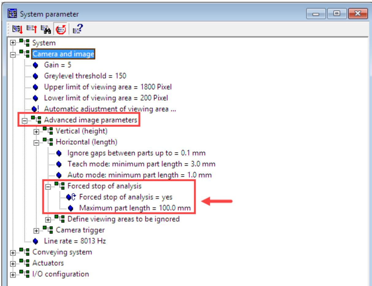
The number of "aborts" can be configured so that this state does not occur permanently. E.g. when a part gets stuck in the in the viewing area of the checkbox.
