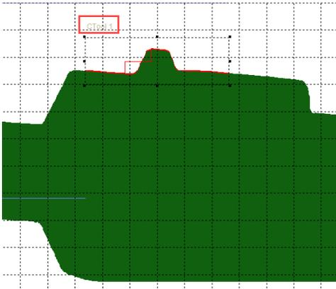
In this example, the tool determines the height difference in a defined section of the contour. If the collar is missing, then the height difference is different from the sample parts. This could be evaluated.
