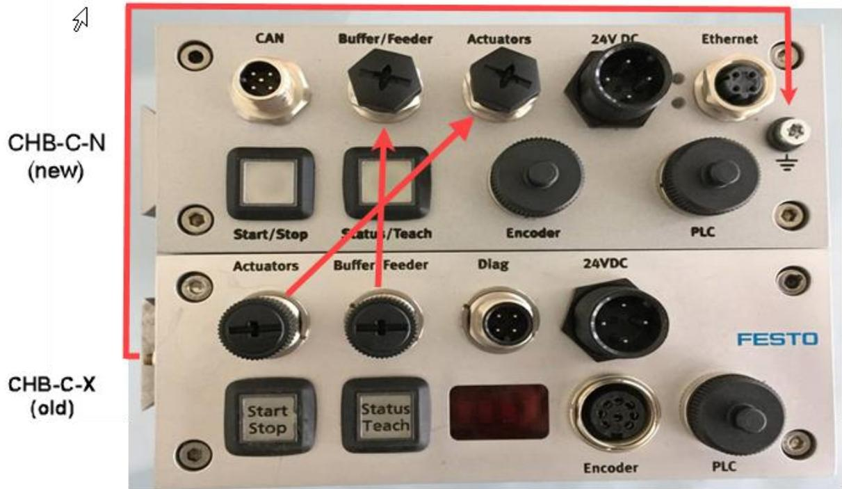
The earth connection point PE is located on the front panel of the new device. Here it has to be checked whether the existing length of the PE cable is sufficient. If necessary, the cable must be adapted.
