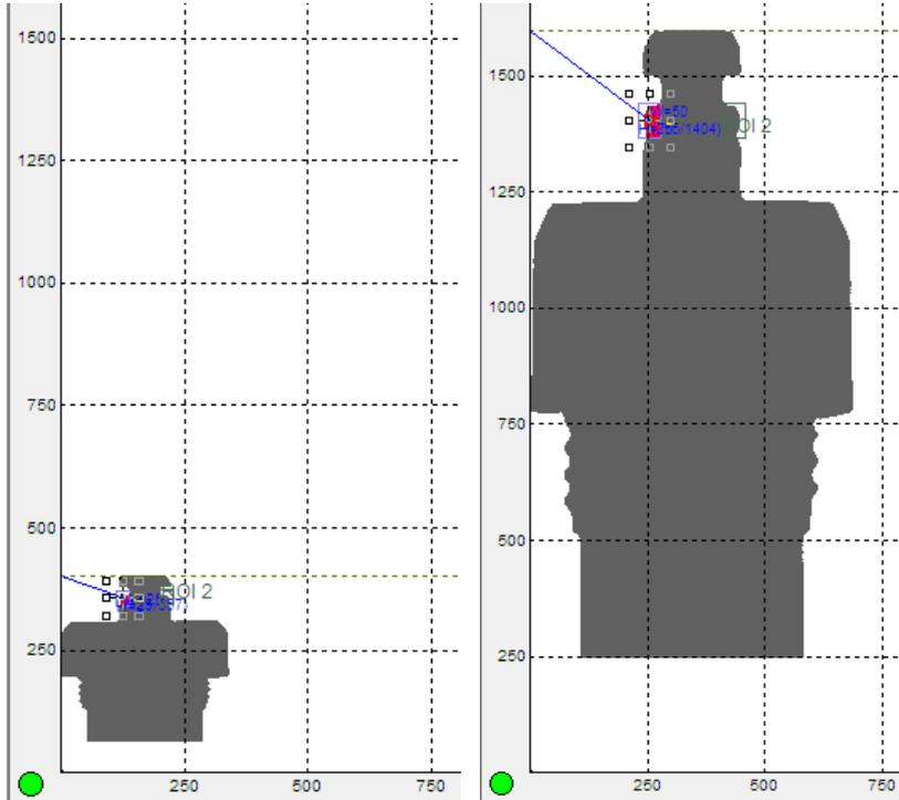
On the left, with low resolution, the presence of an O-ring with approx. 300 pixels is checked. With increased resolution in both directions and with adjustment of position and size, the ROI is checked with approx. 2200 pixels. This makes the evaluation more reliable and stable.
