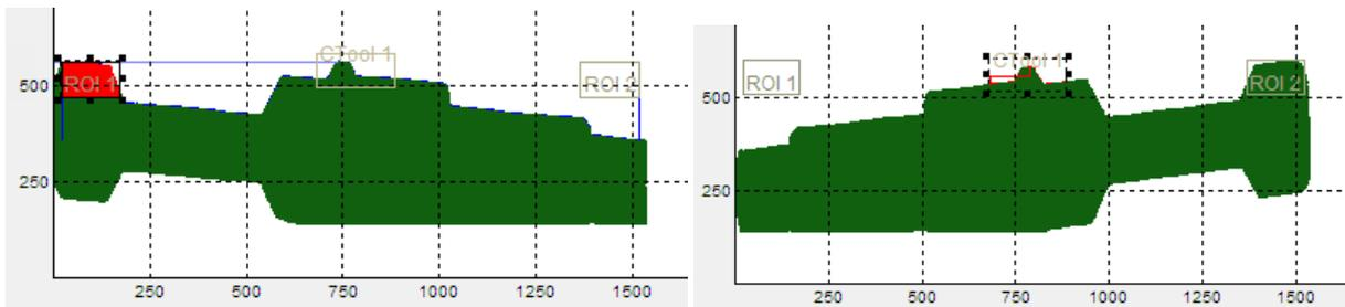
The position orientation is done by 2\*ROI. These are placed symmetrically at the front and rear of the part. In each position one ROI is "filled" the other ROI is "empty" So the position is clearly defined. The presence of the collar in the middle is checked by the Ctool. If the collar is missing, the Ctool creates different values.
