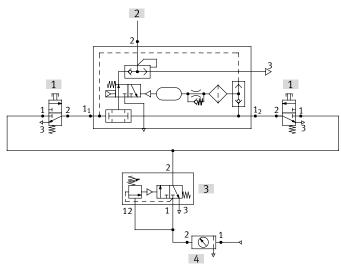
[1] Front panel valve with pushbutton actuator, e.g. SV-3, T-30
