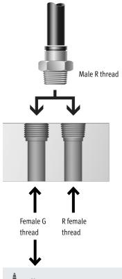
If male R threads are combined with female G threads, leakage can occur if the female G thread was not manufactured cleanly or if it is not within permissible tolerances. In this case additional sealing, e.g. using a sealing band, is required.
