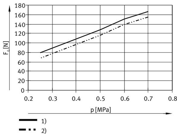
The gripping force refers to one gripper jaw, without mounted gripper fingers.
