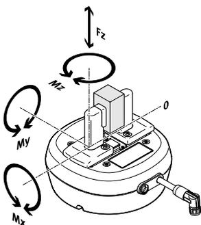
The indicated permissible forces and torques refer to one gripper jaw. The indicated values include the lever arm, additional applied loads due to the workpiece or external gripper fingers and acceleration forces occurring during movement. The zero coordinate line (gripper jaw guide) must be taken into account when calculating the torques.
