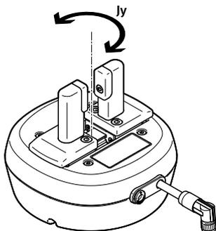
Mass moment of inertia of the gripper in relation to the central axis, with pre-mounted gripper fingers, HAFH-B30-16-45-N, with no load.
