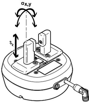
The gripper has a ball guide, which eliminates any possible backlash between the gripper jaws and the housing. The backlash values listed in the table have been calculated based on the traditional accumulative tolerance method.
