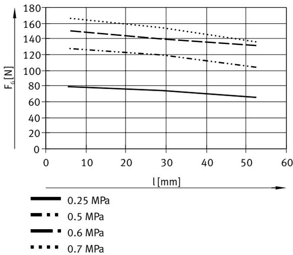
The gripping force was measured with the gripper fully open and gripping a work-piece with a width of 16 mm.
