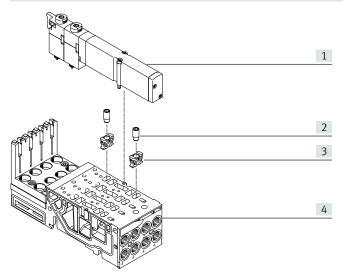
The fixed flow restrictor can be used to permanently set the exhaust flow rate in ducts 3 and 5. To be able to screw the restrictor into the sub-base, the retaining bracket is first pressed into the exhaust openings on the subbase as far as the stop.
