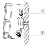
The valve terminal MPA is hooked onto the DIN rail  $\rightarrow$  arrow [1]. The valve terminal MPA is then swivelled onto the DIN rail and secured in place with the clamping piece  $\rightarrow$  arrow [2]. The following MPA mounting kit is required for DIN rail mounting of the valve terminal:
