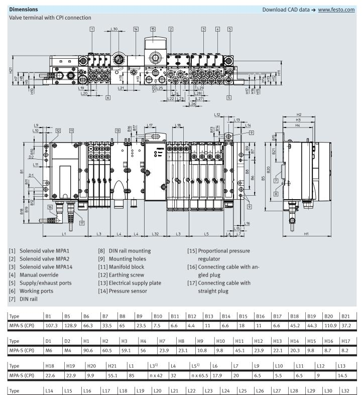
1) n = number of sub-bases (with MPA1, width 10 mm and MPA14, width 14 mm, max. 4 valve positions on sub-base; with MPA2, width 20 mm, max. 2 valve positions on sub-base)
