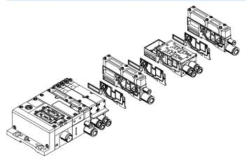
The modular design of the MPA enables outstanding flexibility right from the planning stage and offers maximum ease of service in operation. The system consists of sub-bases and valves.
