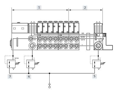
Sub-base with pressure zone separation in duct 1 and duct 3/5
