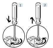
Press in the plunger of the MO with a pointed object or screwdriver until the valve switches and then turn the plunger 90° clockwise until the stop is reached.
