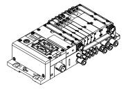
An integrated bus node manages communication with a higher-order PLC. This enables space-saving pneumatic and electronic solutions to be implemented. Valve terminals with fieldbus interfaces can be configured with up to 16 sub-bases. In combination with the MPA1 or MPA14 and 8 solenoid coils per sub-base, up to 128 solenoid coils can thus be controlled. An MPA2 with 4 solenoid coils per sub-base can actuate 64 solenoid coils.
