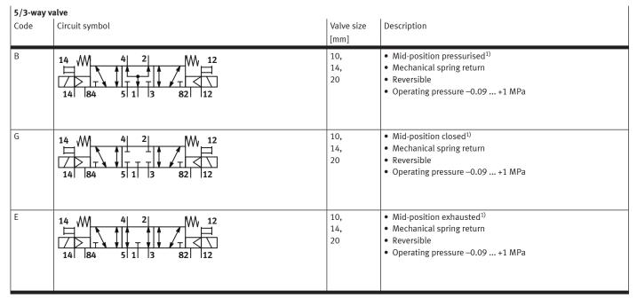
1) If neither solenoid coil is energised, the valve is moved to its mid-position by spring force.
