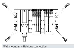
The MPA valve terminal is screwed onto the mounting surface using four M4 or M6 screws. The mounting holes are on the pneumatic interface and on the right end plate. Optional mounting brackets are also available.
