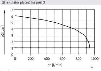
Supply pressure 10 bar, regulated pressure set at 6 bar
