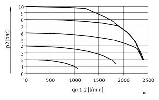
Flow rate qn from 2 → 3 as a function of output pressure p2 VPPM-8TA-...-OL2H-... (2 bar)
