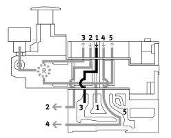
The reversible B regulator splits the supply air in duct 1 and regulates the pressure upstream of the valve in duct 3 (the unregulated pressure from duct 1 is in duct 5). The regulated air is then routed to duct 2. The valve is thus operated in reverse mode. During exhausting, the exhaust flow in the valve is from duct 2 to duct 1 and the air is returned to duct 3 via the intermediate plate.
