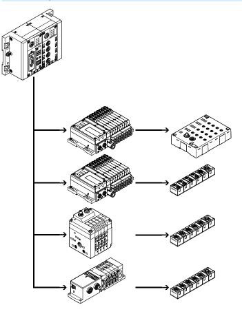
Valve terminal for installation system CPI:
