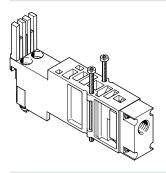
This vertical pressure supply plate enables an individual valve to be supplied with individual operating pressure independently of the operating pressure of the valve terminal. The exhaust and pilot air supply of the valve are still provided via the central ports of the valve terminal.
