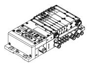
With controllers that are integrated in the Festo valve terminals, stand-alone control units to IP65 without control cabinets can be set up. In the slave operating mode, these valve terminals can be used for intelligent preprocessing and are therefore ideal modules for designing decentralised intelligence. In the master operating mode, terminal groups can be designed with many options and functions that can autonomously control a medium-sized machine/system. → Internet: cpx
