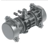
With the single-acting quarter turn actuator, the incoming compressed air moves the pistons in one direction. This generates the torque of the actuator. The springs built into the actuator are pre-tensioned at the same time. This spring force generates the torque in the opposite direction of rotation when the pressure chambers of the actuator are exhausted. This causes the process valve to move to the required initial position.
