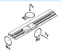
If the drive is simultaneously subjected to several of the indicated forces and torques, the following equation must be satisfied in addition to the indicated maximum loads:
