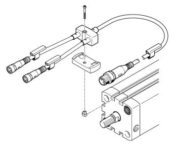
The distributors NEDY have a throughhole suitable for an M2 screw on the distributor housing.
