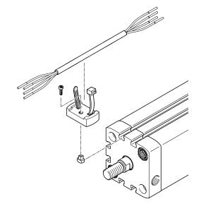
The mounting kit guarantees secure mounting in T-slots from Festo. The geometry of the retaining bracket and of the slot nut are precisely adapted to these T-slots.
