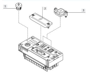
Covers are inserted/screwed into or placed/screwed onto unused connections/openings.
