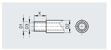
Before the plastic tubing PAN-VO can be inserted into the push-in fitting QS-VO, the tubing's PVC sheath must be cut by length X.
