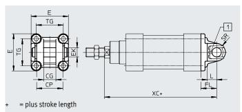
[1] The pivot pin is secured against rotation with a spring pin.
