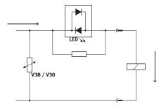
Each solenoid coil is protected with a spark arresting protective circuit as well as against polarity reversal.
