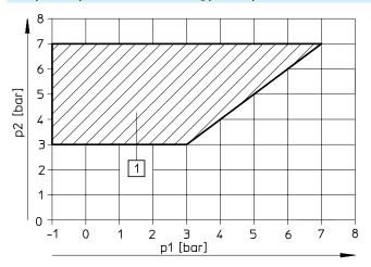
[1] Operating range for valves with external pilot air supply
