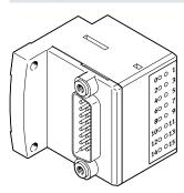
With this electrical connection variant, all valves are controlled centrally via the 15- and 26-pin connector plug. The electrical connection is located on the left-hand side.
