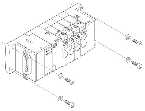
Mounting holes for screws M3
