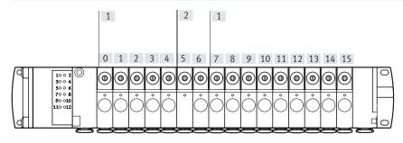
[1] Single solenoid valves occupy one valve position
