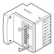
With this electrical connection variant, all valves are controlled centrally via the 20-pin connector plug.
