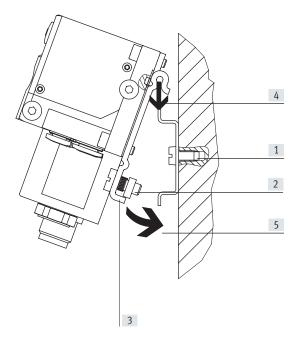
The valve terminal CPV-SC is attached to the H-rail → arrow [4]. It is then swivelled onto the H-rail and secured in place with the clamping component → arrow [5].
